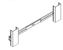
Mounting the rear ear bracket to rear side of rail. Adjust the rear ear bracket according to depth of your cabinet. If a screw hole is available, secure ear bracket to outer rail with a M4 screw. If only open slot is available, secure rear ear bracket with outer rail with both screw at front and hex nut at other side. Do not tighten screw yet. **6** Attaching center rail to right side of shelf. Make sure all 4 screw holes are aligned. Secure center rail to shelf with (4) M4 screws.
