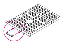
**9** Align center rail with outer rail in the cabinet. Push shelf in until you hear the metal tap click. Push down the metal tap on the center rail to continue. You might encounter a little resistance when push in. That is normal.
