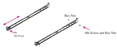
on to cabinet. Tighten all M4 screws on the outer rail.
